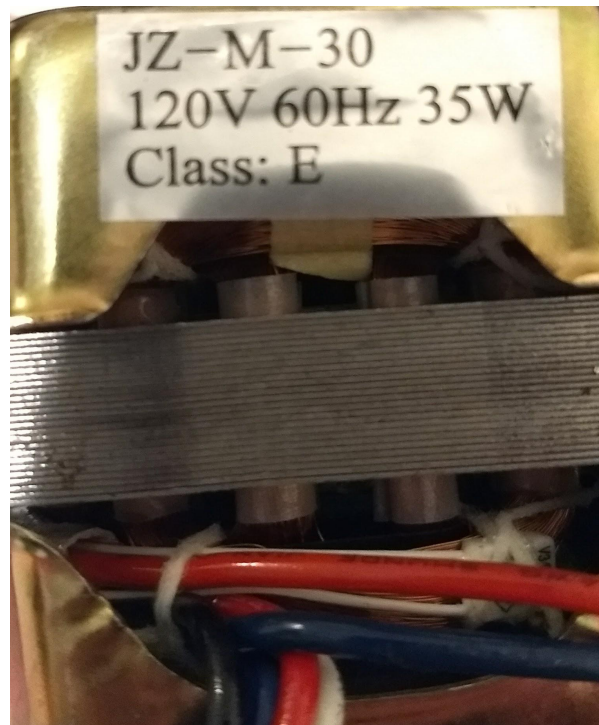
Figure 6-3: Fan Motor Connecting Wires
