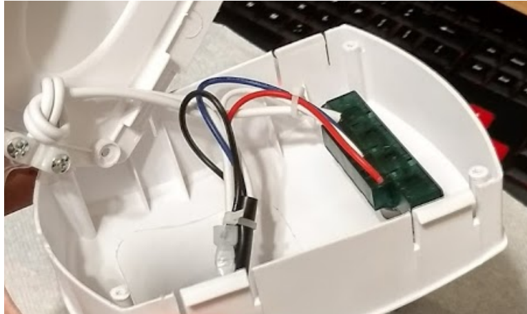
Figure 6-8: Oscillating Fan Switch Assembly
